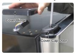
23. After disassembling Grommet and Cap wire at the left side, assemble them into the right side.
